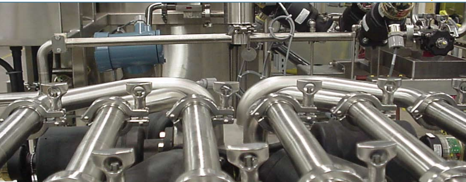
ITT chromatography valve assembly connecting the chromatography column to the process piping
